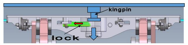
(The king pin automatically opens the catch during loading)
