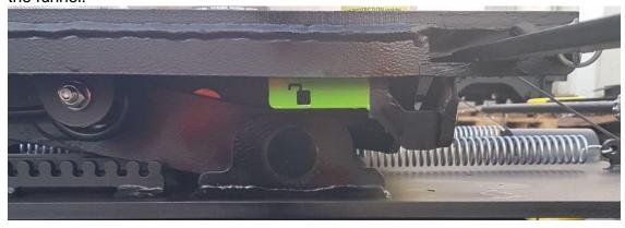
As long as the indicator (red or green > dependant on the customer) is visible, the king pin is not in the funnel. Not the indicator is not longer visible, is the kingpin situated in the funnel.
