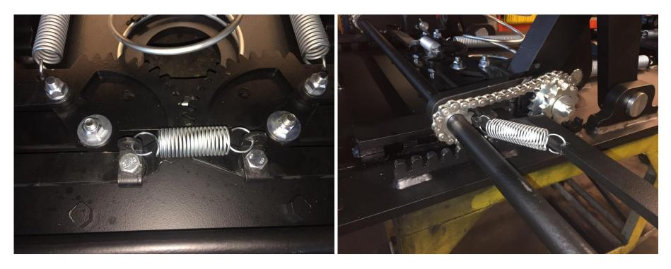
Chains may be sprayed with a chain spray. CAUTION: DO NOT APPLY GREASE!
