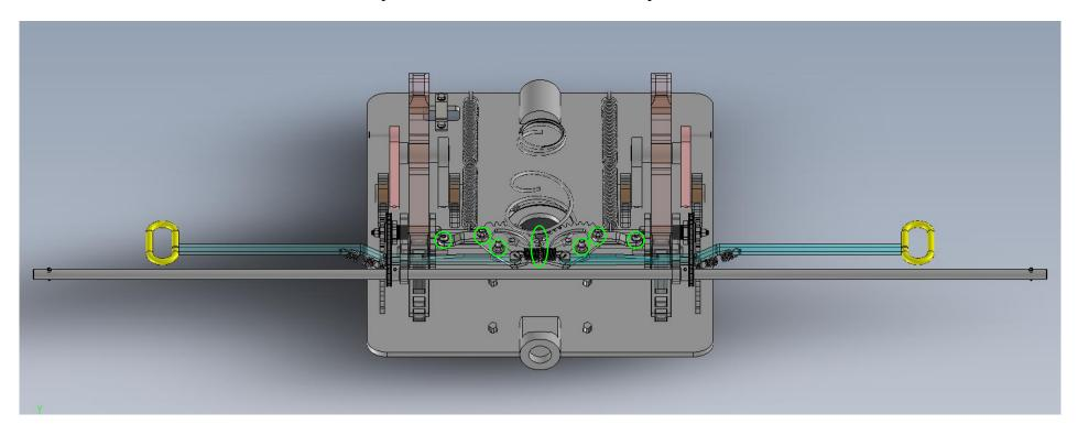
The marked areas are to be sprayed with spray oil during initial operation and maintenance. Following this, lubricating oil is suggested. > see table on page 4
